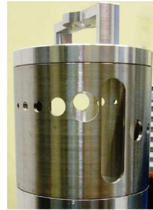
Figure 3: Beam diameter reduction. The cylinder has different diameters hole on its wall. Their position can be set with a stepper motor.
