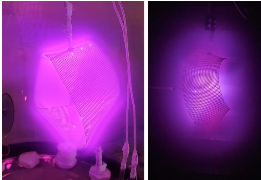
Fig. 5. Plasma discharges with a Möbius electrode. (a) UAIC – Bell shape vacuum chamber, anode at right, (b) UIBK – anode is the chamber
