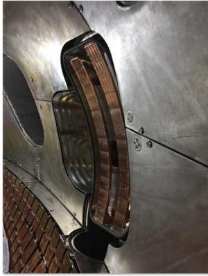
Fig. 1. Photo of two straps antenna inside vacuum chamber W-7X (photo were provided by the Laboratory of Plasma Physics of the Royal Military Academy).
